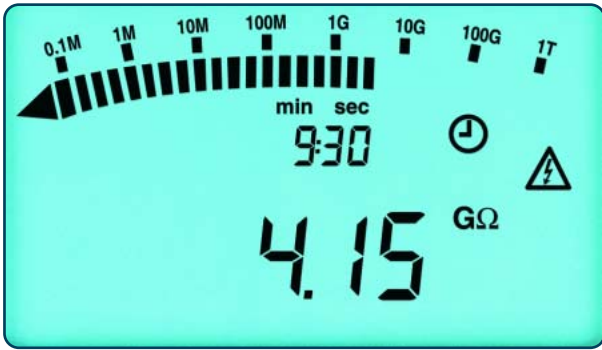
Insulation Resistance Measurement displayed throughout the test. Time or test voltage can be displayed at the press of a button.
