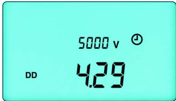
Automatic calculation and display of DD Ratio on request at the conclusion of the test
